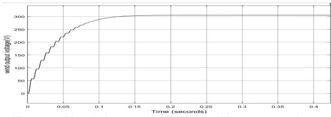
Figure 6: Simulation results of wind turbine output voltage.
