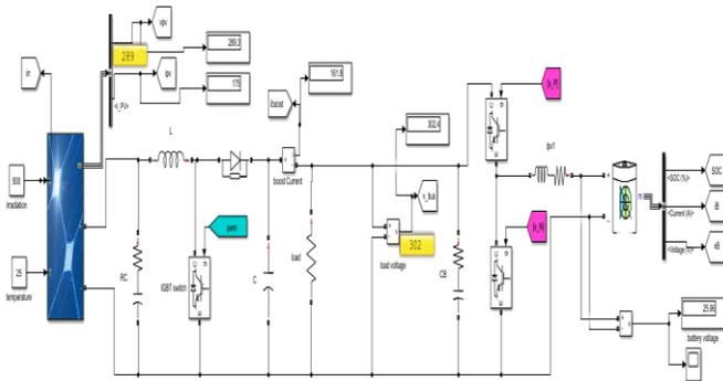
Figure 1: Simulation circuit for integration of solar and battery.
