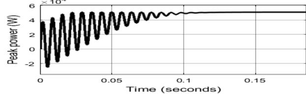
Figure 11: Simulation result of Peak Power without PI Controller.
