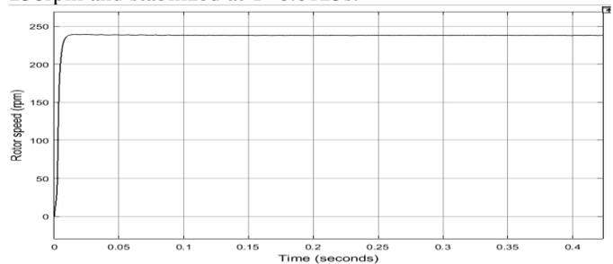
Figure 5: Simulation results of wind turbine rotor speed.
