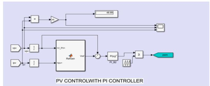
Figure 3: PV control model for MATLAB function to analyze peak power with PI controller.
