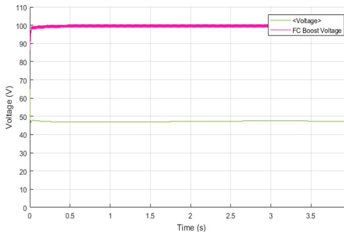
Fig 5: Output Voltage of FC and FC boost voltage
