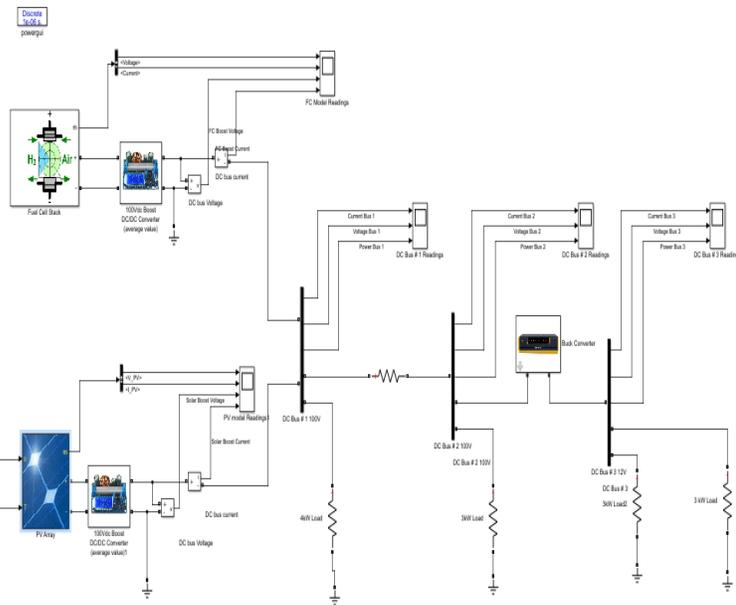
Fig 2: Simulation model of the proposed PV and FC hybrid generation system
