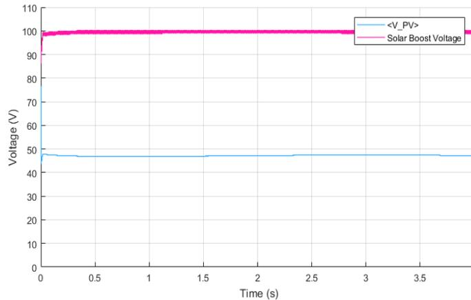
Fig 4: Output Voltage of PV array and Solar boost voltage
