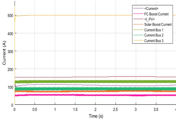
Fig 3: Steady state current at DC buses and generation systems
