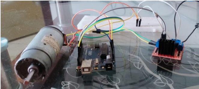
Figure 7. Setup for DC Motor Speed Control
