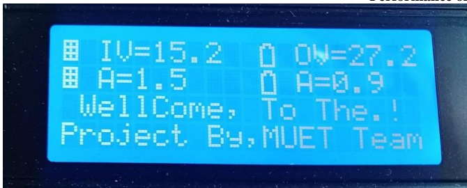
Fig 11: Display module of PV system
