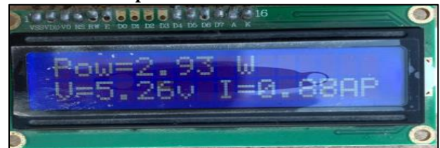
Figure11: LCD displaying of Dual Axis Tracking at 12:00pm
